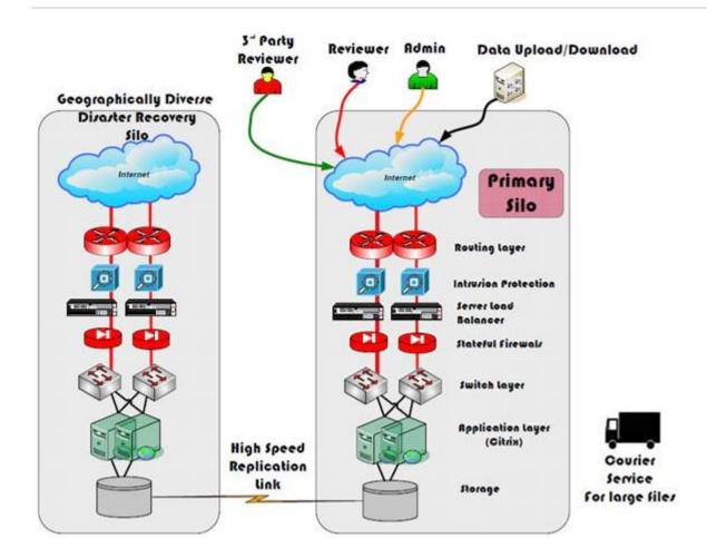
Each LexisNexis Hosted Litigation Solutions customer has its own virtual local-area network (VLAN), allowing only required traffic in and out and granting no access to other customer traffic. Internal firewalls separate the hosted litigation environments from the LexisNexis internal environment and other LexisNexis product offerings. Only LexisNexis staff members directly responsible for supporting Hosted Litigation Solutions are permitted access to the hosted litigation environments.
